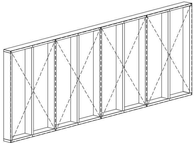
And that's all there is to it ~ one structural wall-panel ready for erection!
