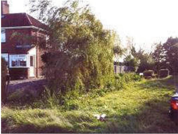
The scene of the "filled-in" pond and old watercourse - note the "willow tree" clue! However the whole area had also been built up with soil 'fill' material as well; leading to the need for piling and a self-supporting floor construction!
